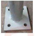
Upon request, it is possible to receive the post with welded base panel (140 x 120 x 8 mm, incl. 4 holes Ø 14 mm). Ground anchoring must be carried out on site (Recommendation: Injection system with Fischer Anchor FIS A / RG M12x260).
