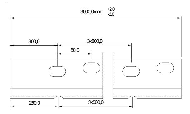
If needed it is possible to drill further suitable holes by yourself to create even smaller rail sections.
